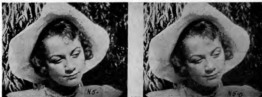
Fig. 5. Photographs of the monitor kinescope images. Photographs from the same frame of a normal 16-mm print. Left, with filters; right, without filters.
